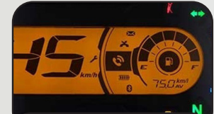
RTMI Displays current mileage of the vehicle in kmpl
